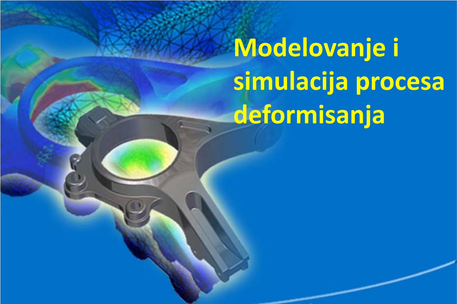
A 3D CAD model of a mechanical part, possibly a bracket or a handle, is shown with a stress simulation. The part is rendered in a dark grey color. The simulation results are displayed as a color map on the part's surface, with green and yellow indicating lower stress levels and red and purple indicating higher stress levels. The background is a blue gradient with a faint, glowing grid pattern.
